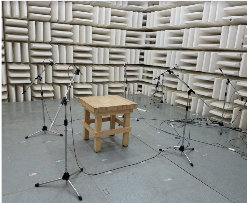
Figure 7: Testing setup at Foxconn CMC anechoic chamber with < 6 dBA background noise
